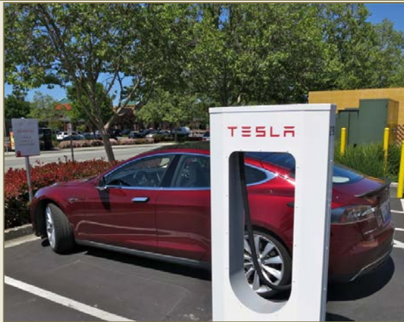
Tesla SuperCharger, 90kw EVSE located in Gilroy, California.
